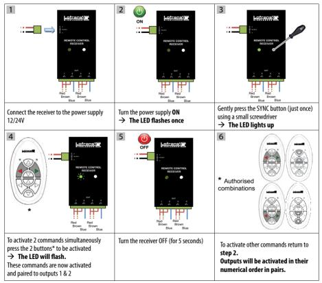
**Note**: Each receiver can handle a maximum of 4 channels: 2 sets of 2 buttons corresponding to receiver outputs (1, 2, 3 and 4). Should the full 8 channels of the transmitter be required, a second receiver is needed.
